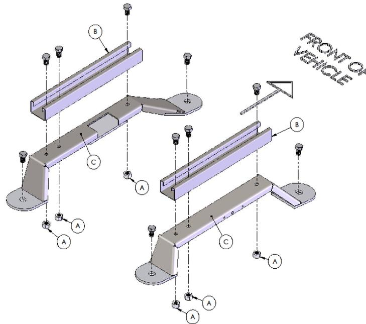
4. Remove the (3) 13mm flange nuts (A) from each side of the seat that hold the slider frames (B) to the original floor brackets.
